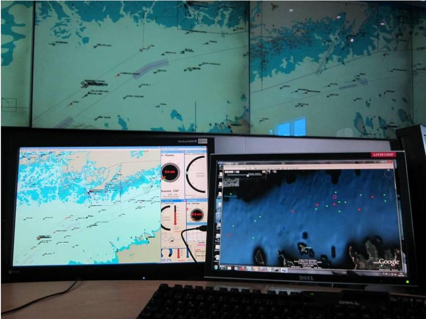
**Figure 2 One of the GOFREP work stations at Gulf of Finland Traffic Centre. The IWRIS system is displayed on the screen to the right.**
